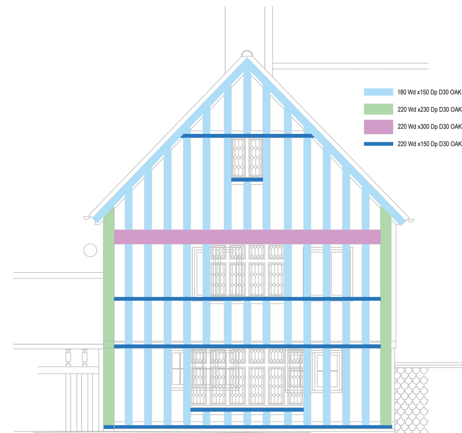
REBUILT ELEVATION TIMBER SIZES
