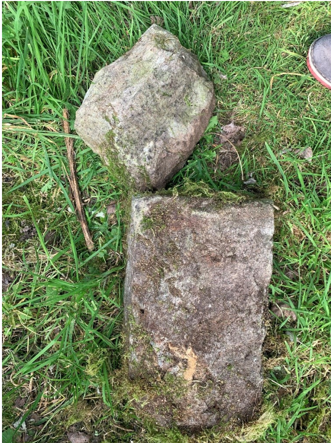
Fig.1 (Left) Sample of Kentish Ragstone on site to be used for repairs and plinth to new gable wall. This will be cleaned off and selected ready cut stones will be used.
