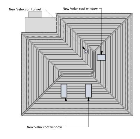
Proposed Ground Floor Plan Scale: 1:100 Proposed Lower Ground Floor Plan Scale: 1:100 Proposed Roof Plan
