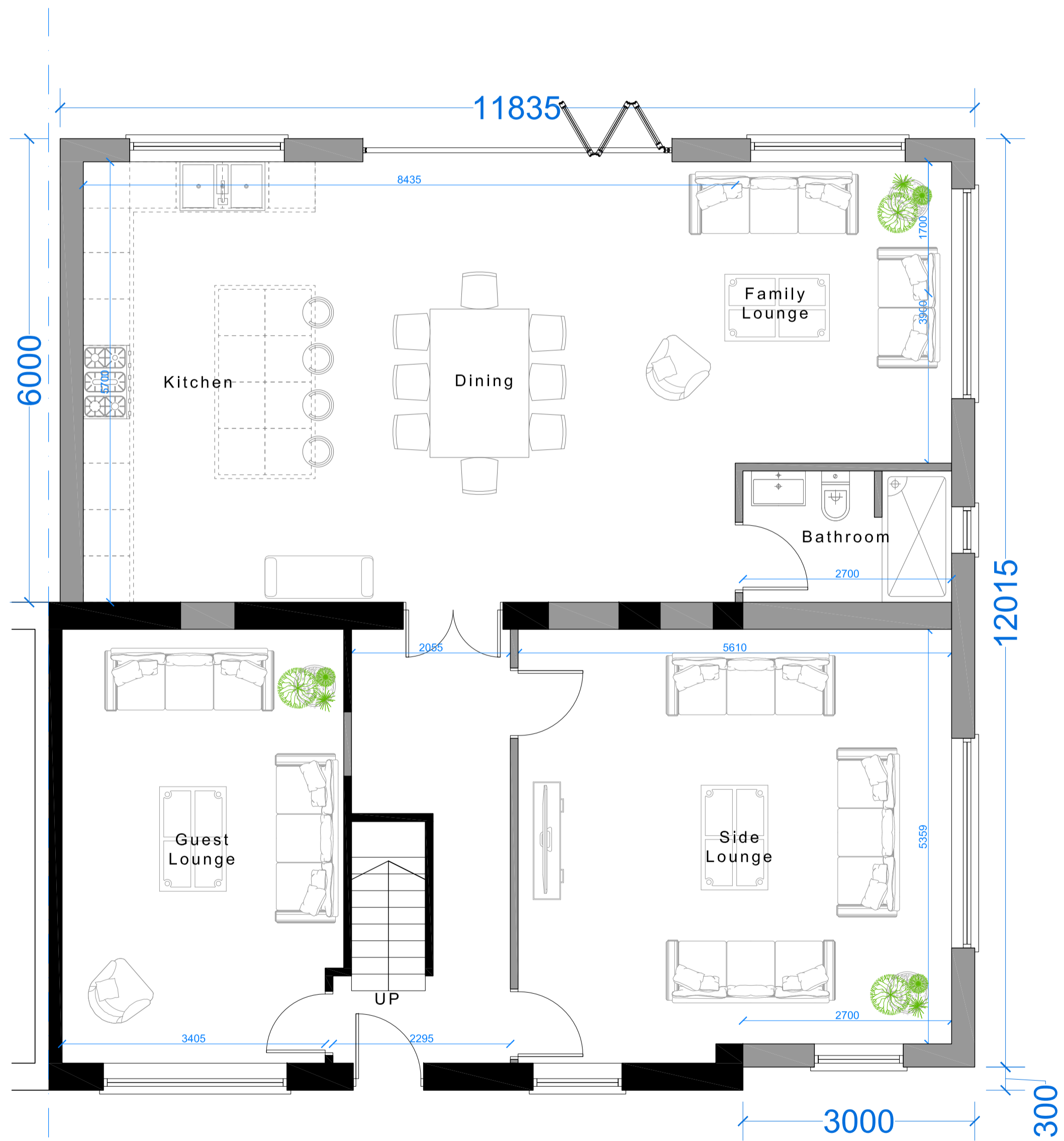
PROPOSED GROUND FLOOR PLAN Scale 1:50@A1
