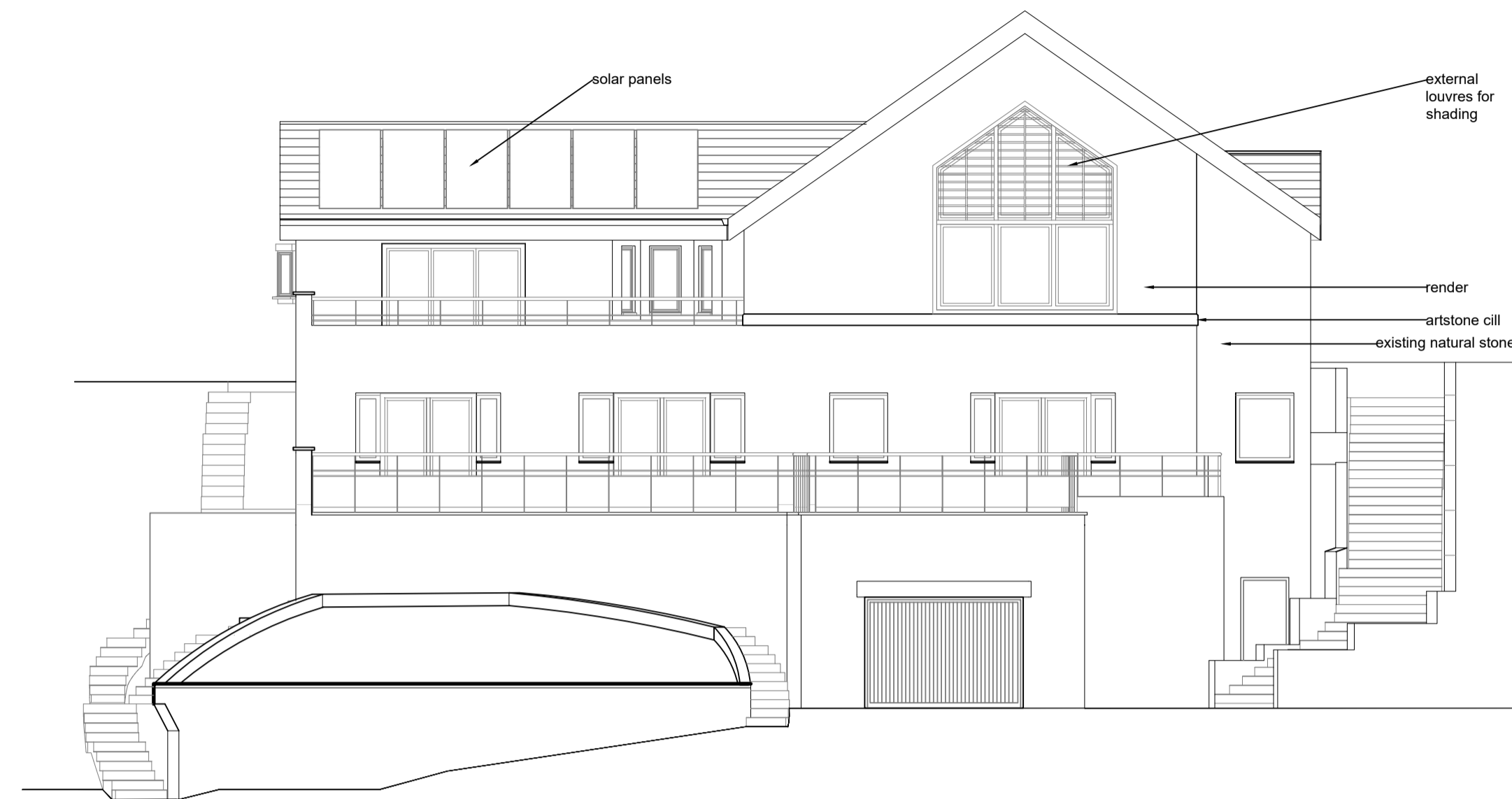
SOUTH WEST ELEVATION 1:100
