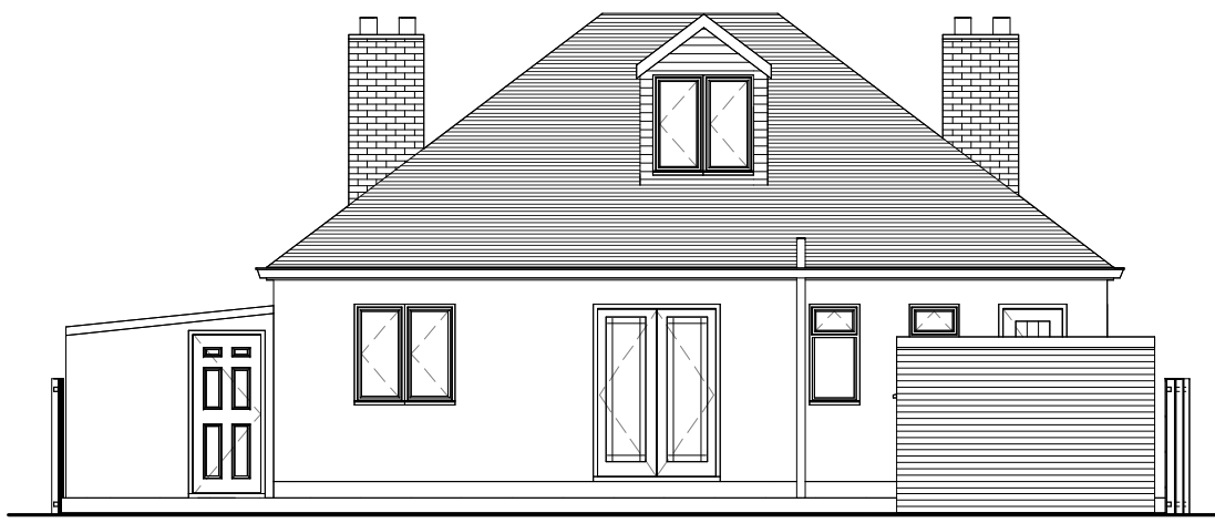
Existing Rear Elevation 1 : 100
