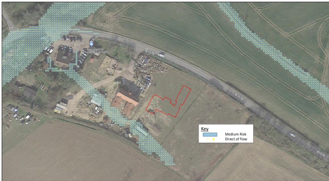
Figure 7- Detailed surface water mapping - Medium Risk Extent including Flow Direction Maximum Velocity (FDMW)
