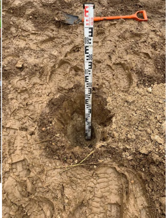
Photographs 1-2 , taken on the 01 st September 2023 showing examples of hand dug trial pits and the nature of the subsoil and topsoil within the soft landscaping of plot 86 (back garden).
