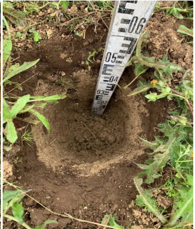
Photographs 5-6 , taken on the 29 th August 2023 showing examples of hand dug trial pits and the nature of the subsoil and topsoil within the soft landscaping of plot 93 (front and back garden).
