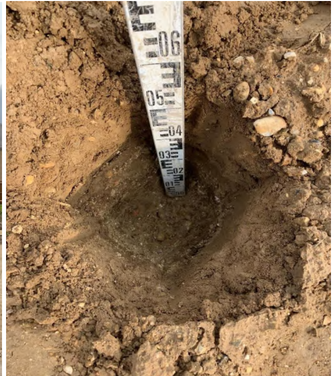
Photographs 3-4 , taken on the 29 th August 2023 showing examples of hand dug trial pit and the nature of the subsoil and topsoil within the soft landscaping of plot 90 (back garden).
