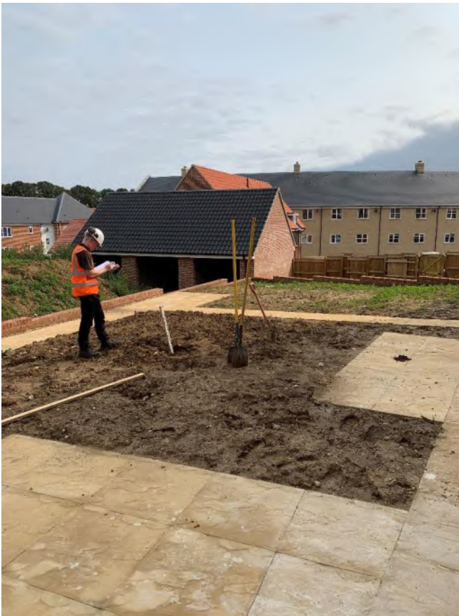
Photographs 1-2 , taken on the 01 st September 2023 showing examples of hand dug trial pits and the nature of the subsoil and topsoil within the soft landscaping of plot 86 (back garden).
