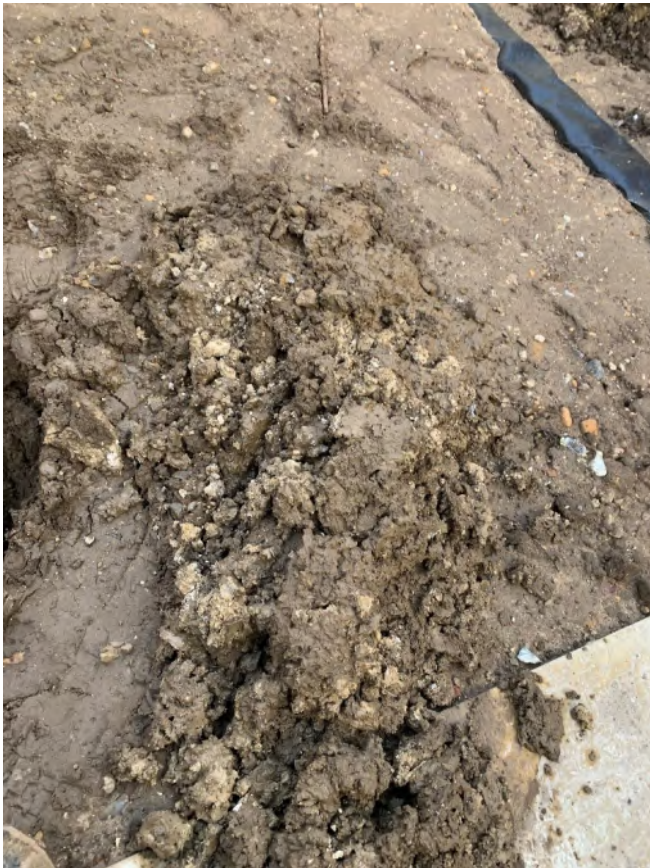
Photographs 8-11 , taken on the 13 th January 2023 showing examples of hand dug trial pits and the nature of the subsoil and topsoil within the soft landscaping of plot 113 (representative of plots 112-117).
