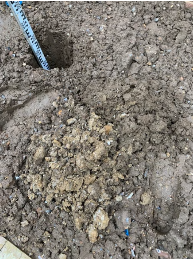
Photographs 1-3 , taken on the 13 th January 2023 showing examples of hand dug trial pits and the nature of the subsoil and topsoil within the soft landscaping of plot 116/117.
