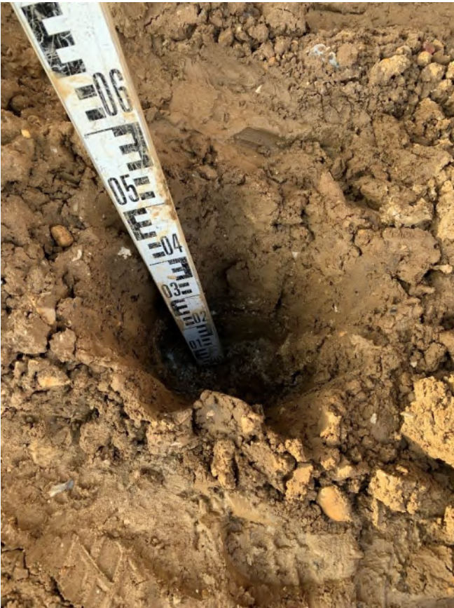
Photographs 12-15 , taken on the 13 th January 2023 showing examples of hand dug trial pits and the nature of the subsoil and topsoil within the soft landscaping of plot 114 (representative of plots 112-117).
