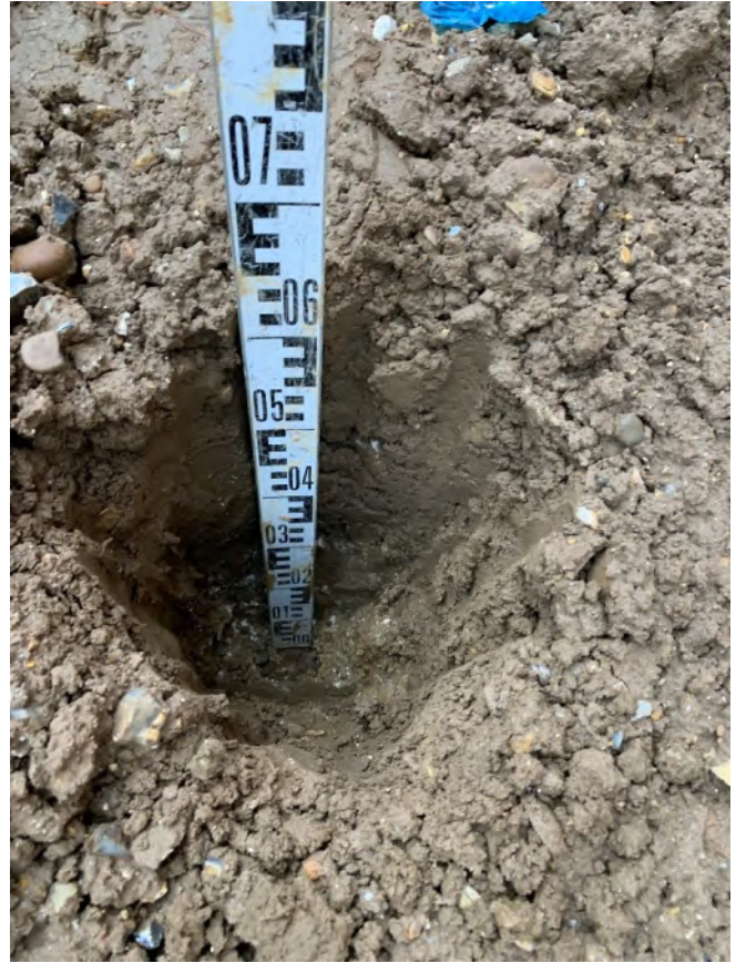
Photographs 1-3 , taken on the 13 th January 2023 showing examples of hand dug trial pits and the nature of the subsoil and topsoil within the soft landscaping of plot 116/117.
