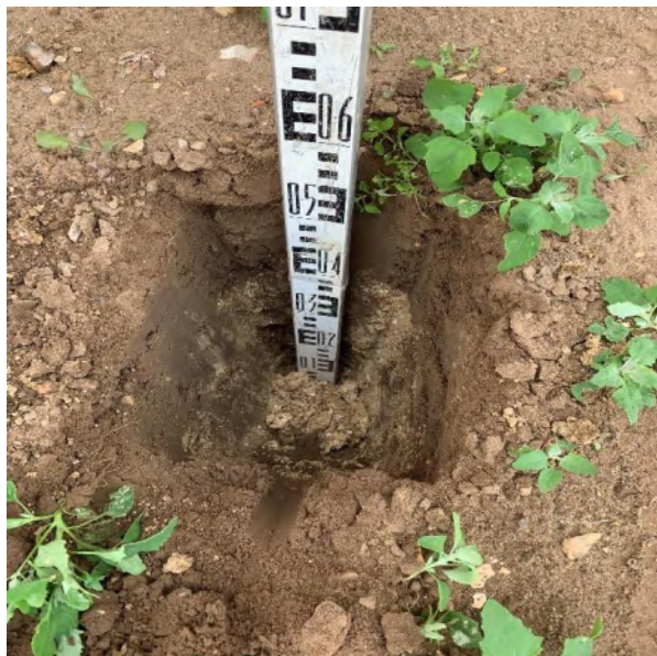
Photographs 1-4 , taken on the 23 rd June 2022 showing examples of hand dug trial pits and the nature of the subsoil and topsoil within the soft landscaping in the back and front garden of plot 58 (representative of plots 57-60).
