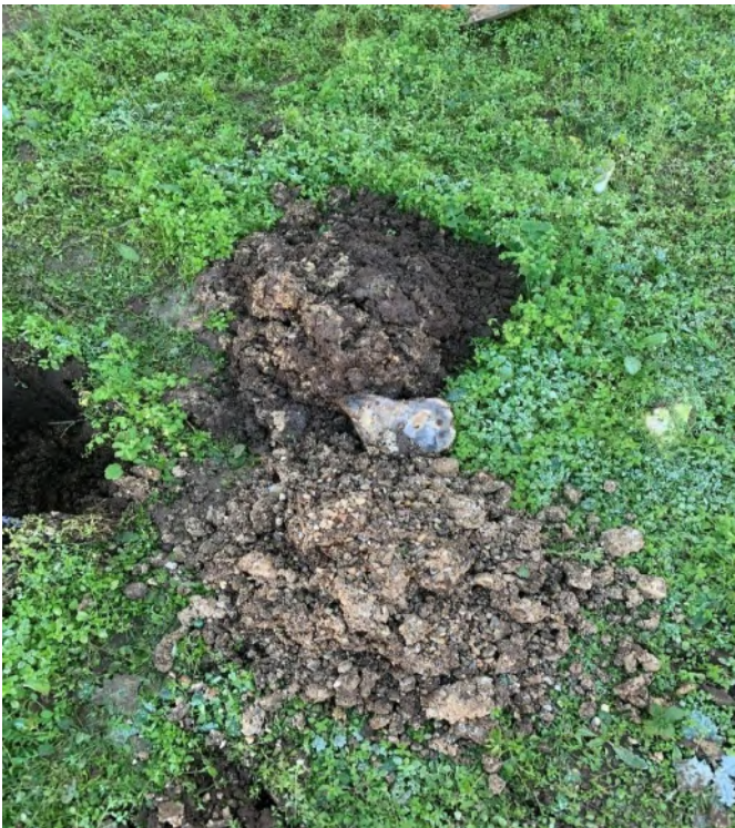
Photographs 1-4 , taken on the 08 th December 2022 showing examples of hand dug trial pits and the nature of the subsoil and topsoil within the soft landscaping of plot 118 (representative of plots 118, 119 and 67-69).
