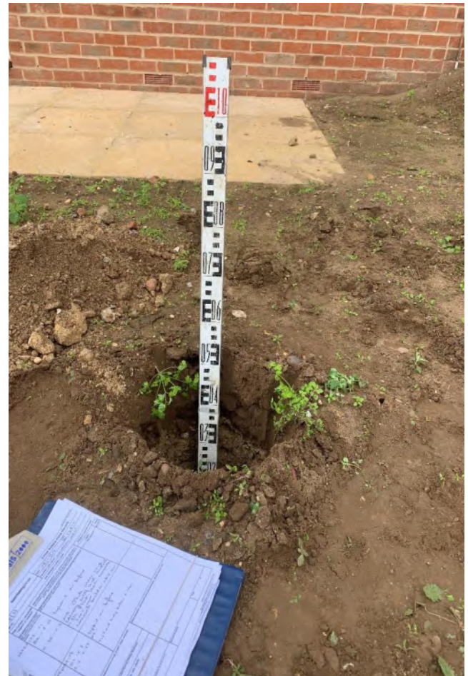
Photographs 5-8 , taken on the 28 th September 2022 showing examples of hand dug trial pits and the nature of the subsoil and topsoil within the soft landscaping of plots 122 and 125 (representative of plots 121-126).
