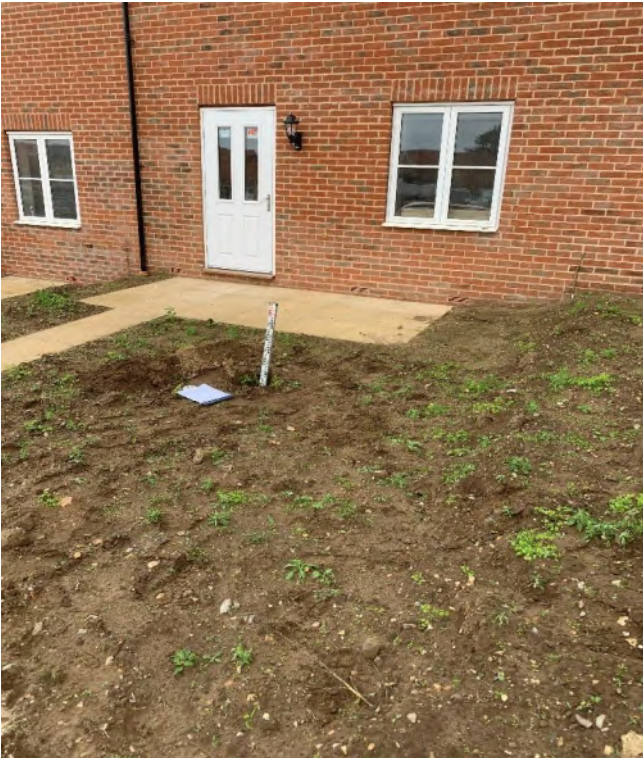
Photographs 5-8 , taken on the 28 th September 2022 showing examples of hand dug trial pits and the nature of the subsoil and topsoil within the soft landscaping of plots 122 and 125 (representative of plots 121-126).
