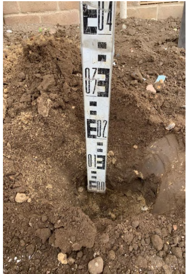
Photographs 9-10 , taken on the 28 th September 2022 showing the topsoil thickness (200mm) within the front gardens of plot 122 (representative of plots 121-123).
