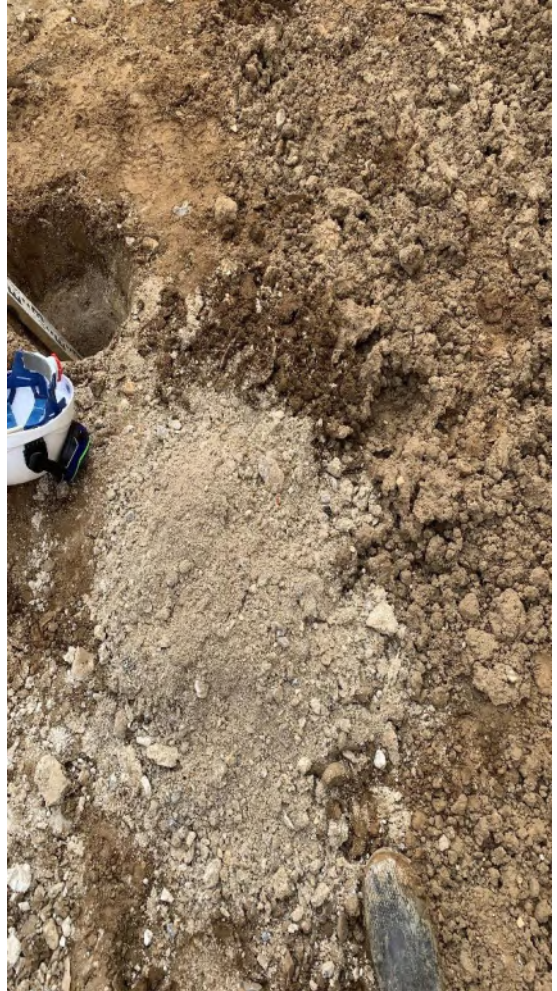
Photographs 9-12 , taken on the 19 th May 2023 showing examples of hand dug trial pits and the nature of the subsoil and topsoil within the soft landscaping of plot 80 (back garden).
