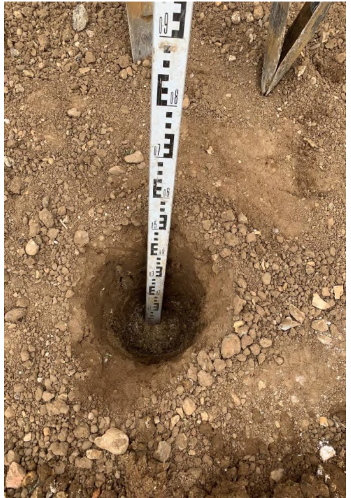
Photographs 1-4 , taken on the 19 th May 2023 showing examples of hand dug trial pits and the nature of the subsoil and topsoil within the soft landscaping of plot 77 (back and front garden).
