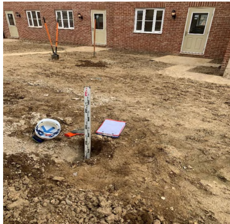
Photographs 9-12 , taken on the 19 th May 2023 showing examples of hand dug trial pits and the nature of the subsoil and topsoil within the soft landscaping of plot 80 (back garden).
