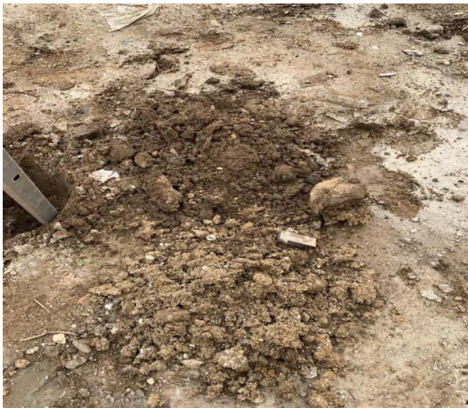
Photographs 5-8 , taken on the 19 th May 2023 showing examples of hand dug trial pits and the nature of the subsoil and topsoil within the soft landscaping of plot 79 (front garden).
