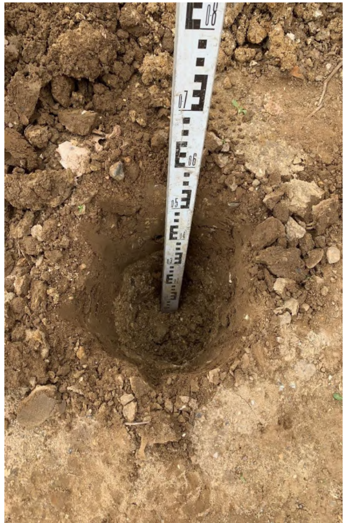
Photographs 5-8 , taken on the 19 th May 2023 showing examples of hand dug trial pits and the nature of the subsoil and topsoil within the soft landscaping of plot 79 (front garden).
