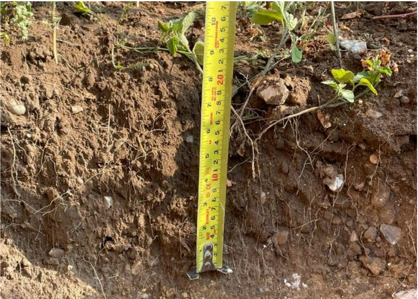
Photograph 9 , taken by HH on the 18 th August 2022 showing thickness of topsoil within plot 198 (representative of plots 197-199) following remedial works.
