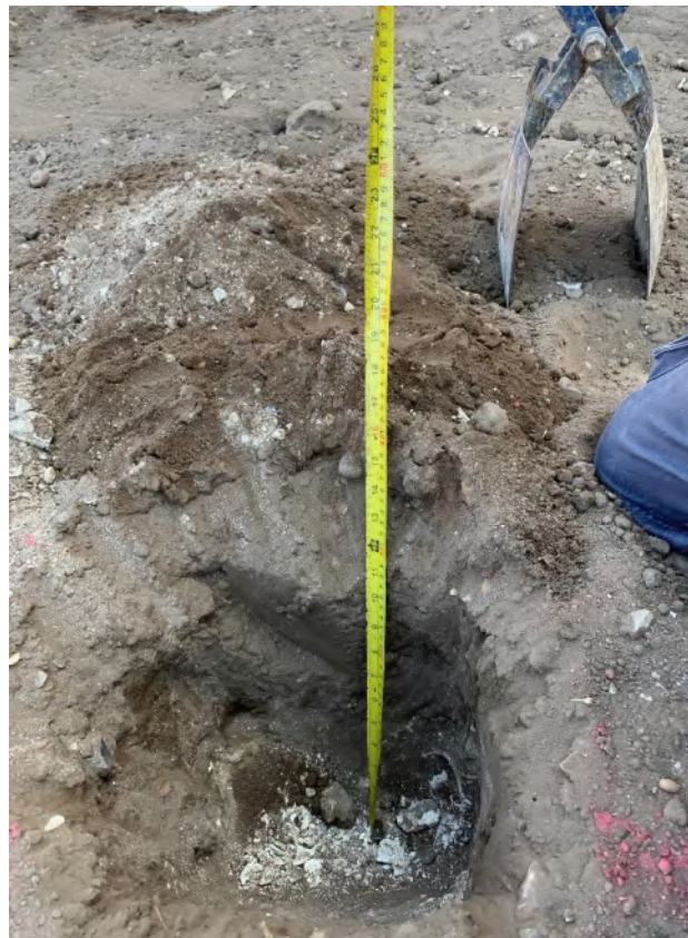
Photographs 1-4 , taken on the 09 th August 2022 showing examples of hand dug trial pits and the nature of the subsoil and topsoil within the soft landscaping of plots 198 and 200-203 (representative of plots 197-199 & 200-203).
