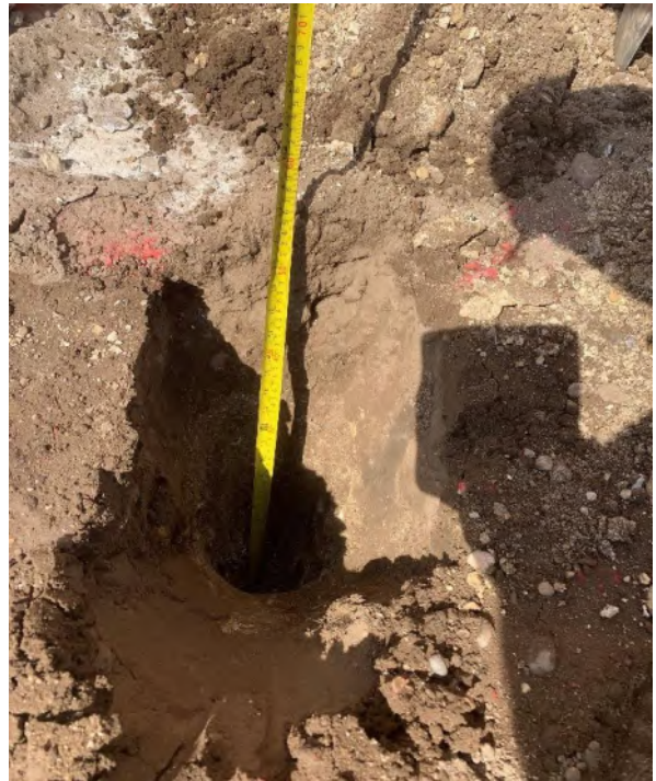
Photographs 5-8 , taken on the 09 th August 2022 showing examples of hand dug trial pits and the nature of the subsoil and topsoil within the soft landscaping of plot 198 (representative of plots 197-199 & 200-203).
