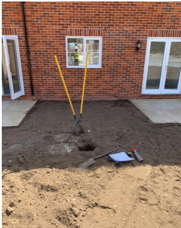
Photographs 1-4 , taken on the 09 th August 2022 showing examples of hand dug trial pits and the nature of the subsoil and topsoil within the soft landscaping of plots 198 and 200-203 (representative of plots 197-199 & 200-203).
