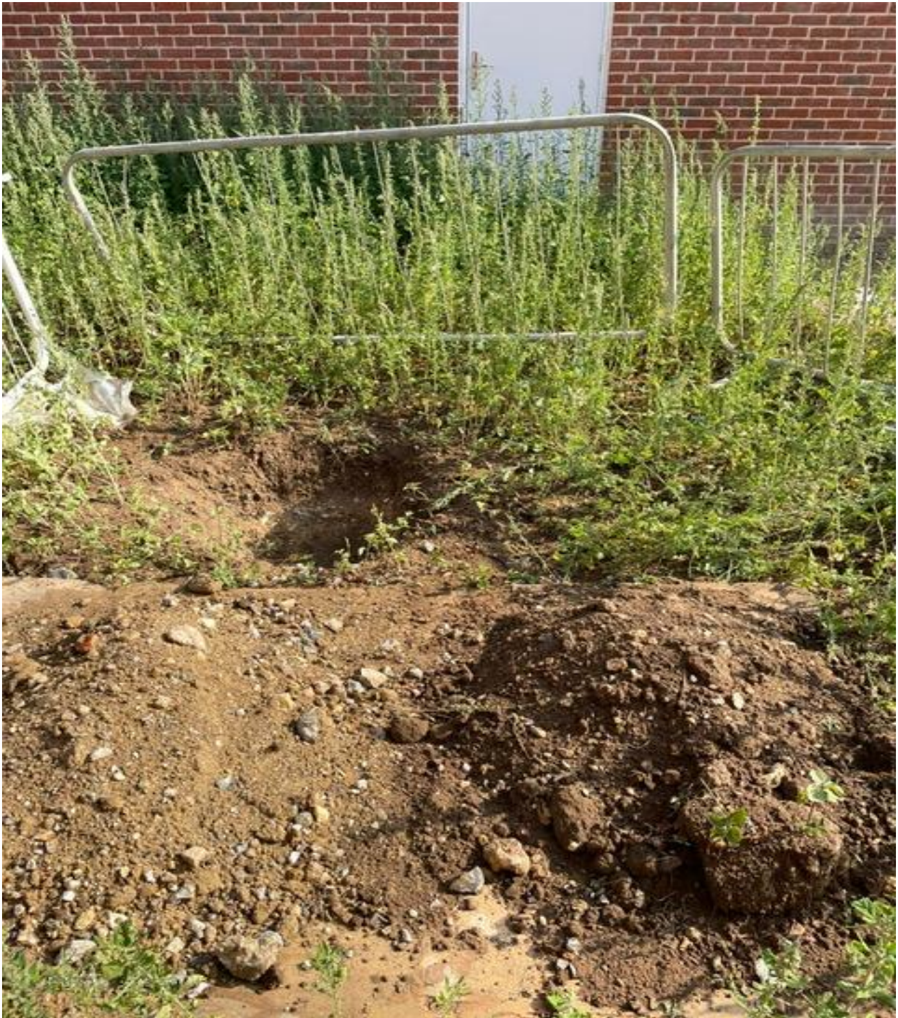
Photograph 8 , taken by HH on the 18 th August 2022 showing the hand dug trial pit and the nature of the subsoil and topsoil within the soft landscaping of plot 96 (very small back garden).
