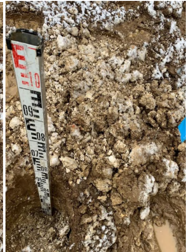
Photographs 12-15 , taken on the 10 th March 2023 showing examples of hand dug trial pits and the nature of the subsoil and topsoil within the soft landscaping of plot 74 (back garden).
