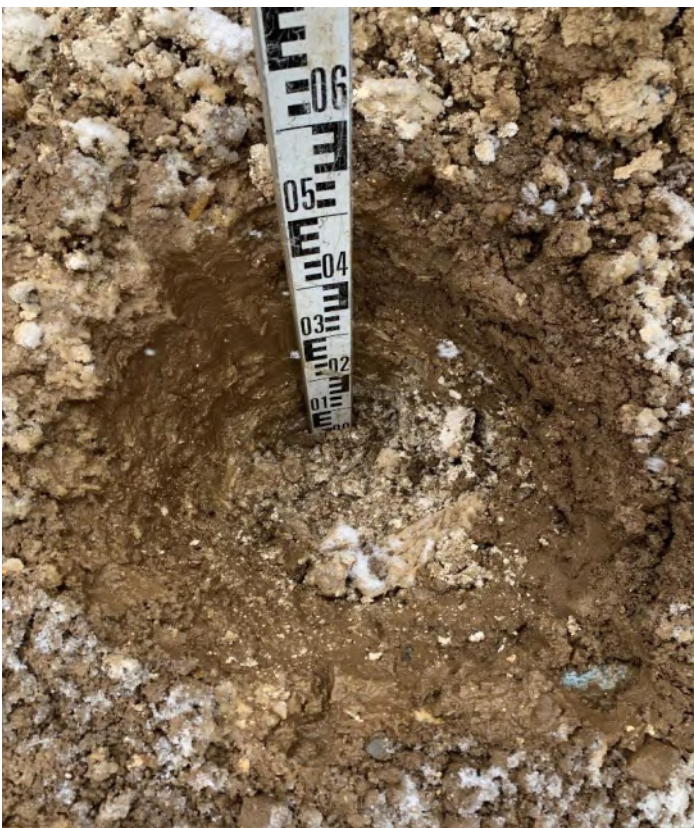
Photographs 12-15 , taken on the 10 th March 2023 showing examples of hand dug trial pits and the nature of the subsoil and topsoil within the soft landscaping of plot 74 (back garden).
