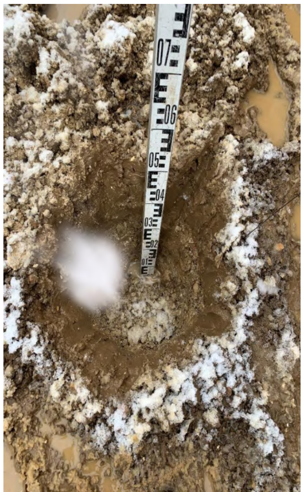
Photographs 4-7 , taken on the 10 th March 2023 showing examples of hand dug trial pits and the nature of the subsoil and topsoil within the soft landscaping of plot 71 (back garden).
