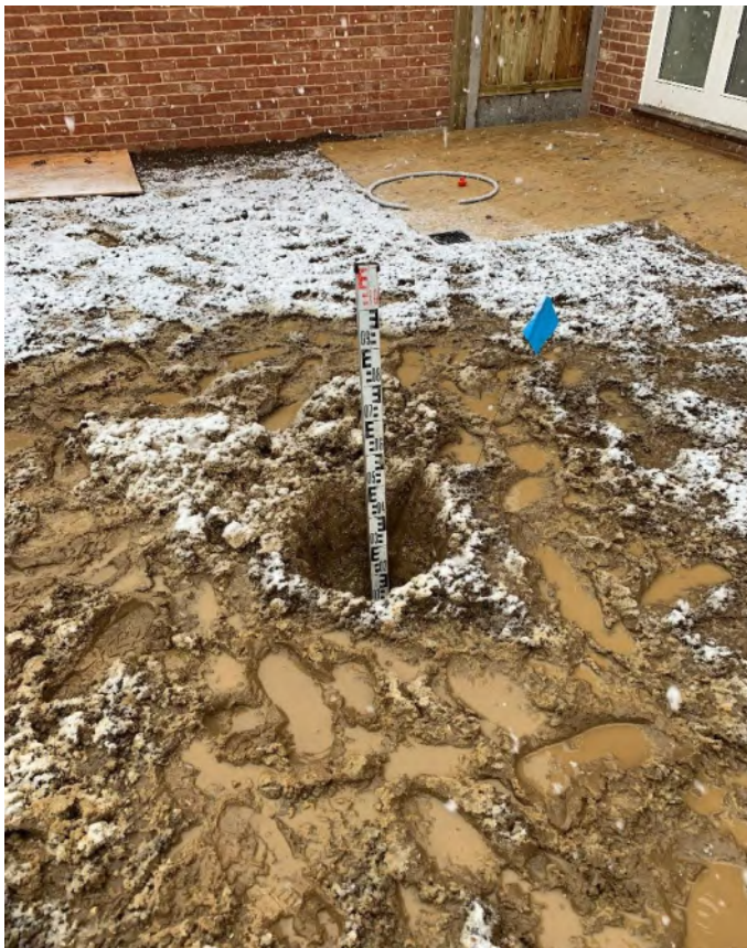
Photographs 4-7 , taken on the 10 th March 2023 showing examples of hand dug trial pits and the nature of the subsoil and topsoil within the soft landscaping of plot 71 (back garden).
