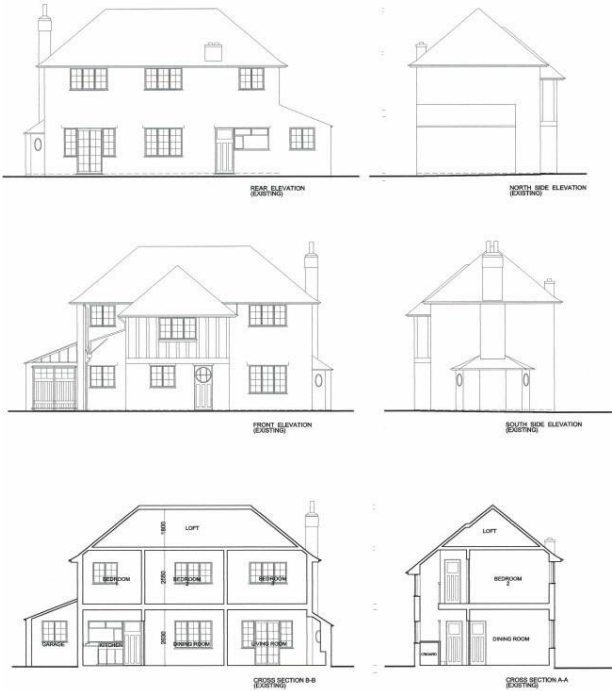
Figure 4. Existing elevations and sections
