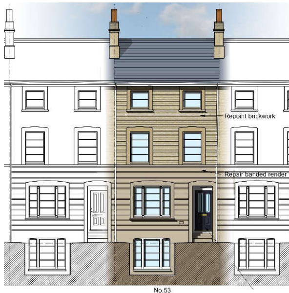
FRONT ELEVATION (incl Lower GF windows)
