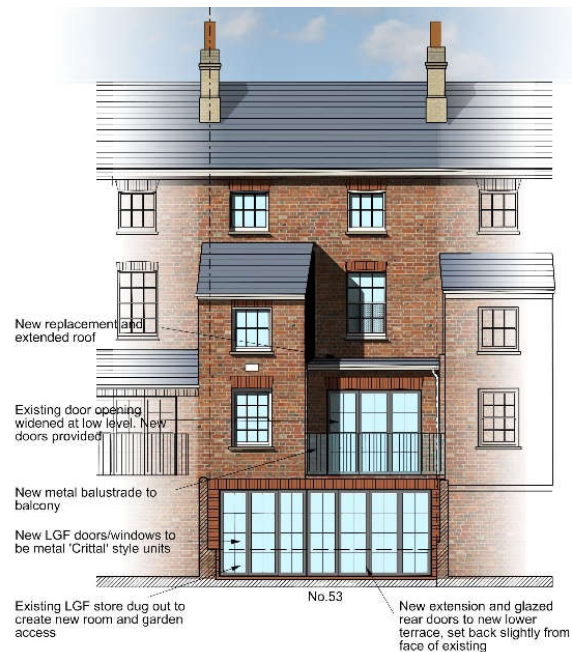
REAR ELEVATION (incl Lower GF windows)
