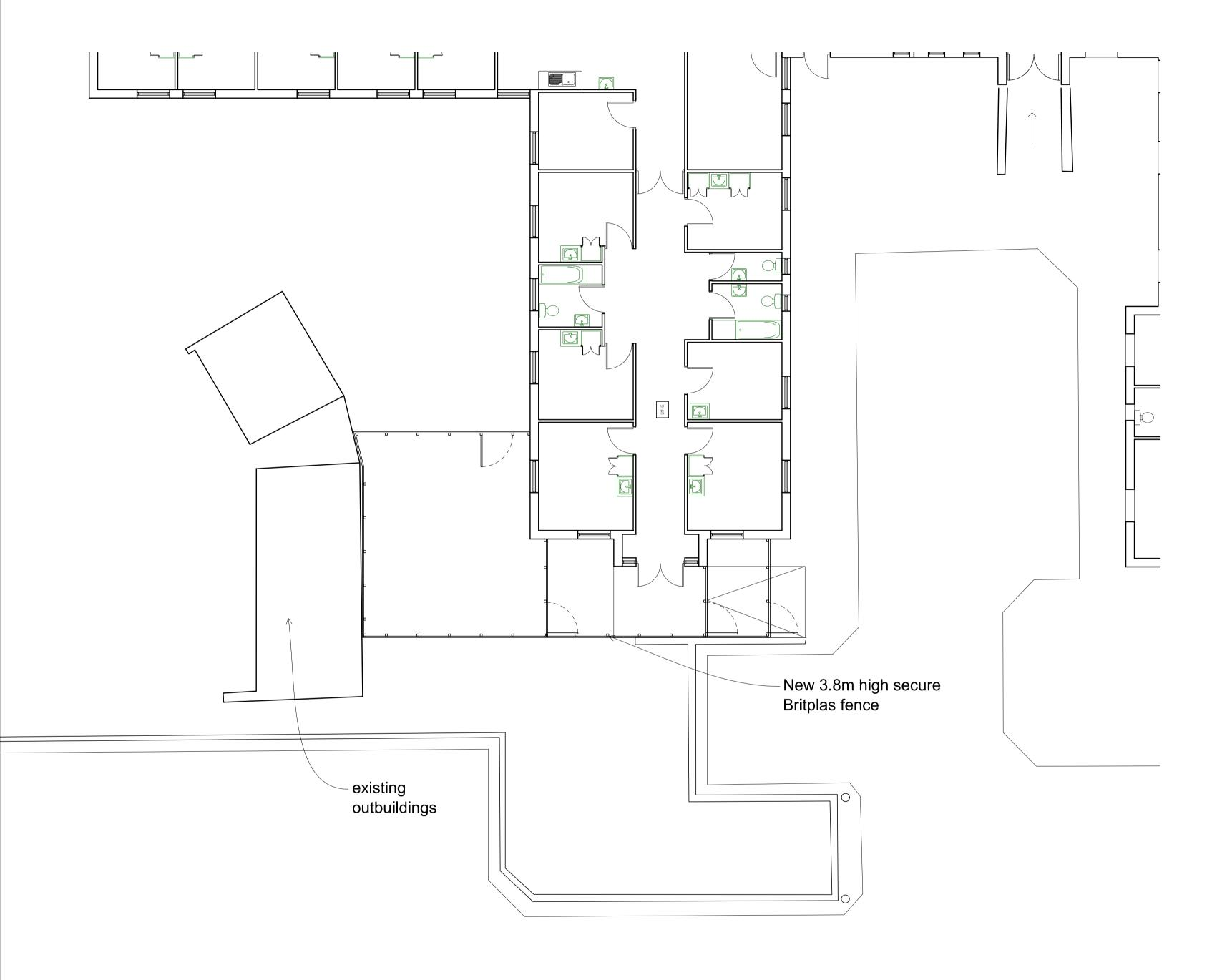
Proposed Plan - new secure fence to front
