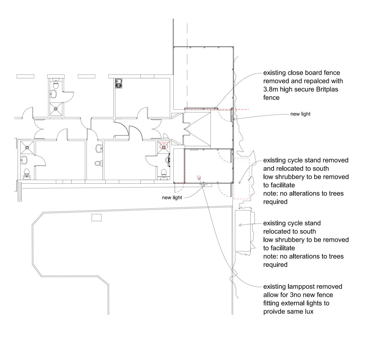
Proposed Plan - new secure fence to 136 unit
