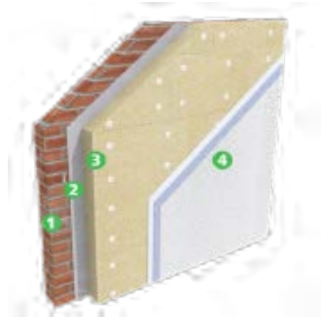
Figure 23. Manufacturer's installation detail IWI to all existing external walls
