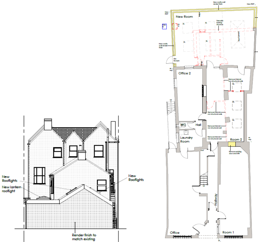
Fig 4 – Proposed Rear Elevation and Ground Floor Plan
