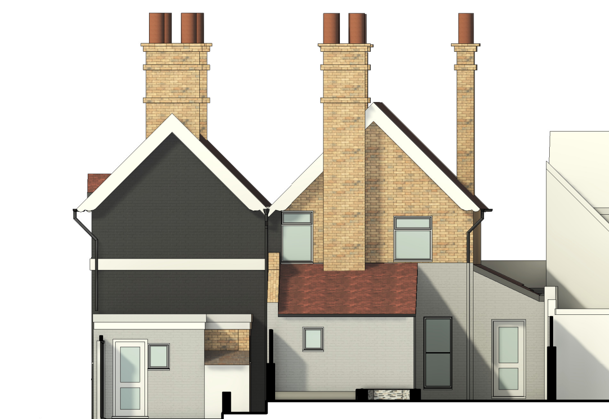
Existing East Elevation 1:100
