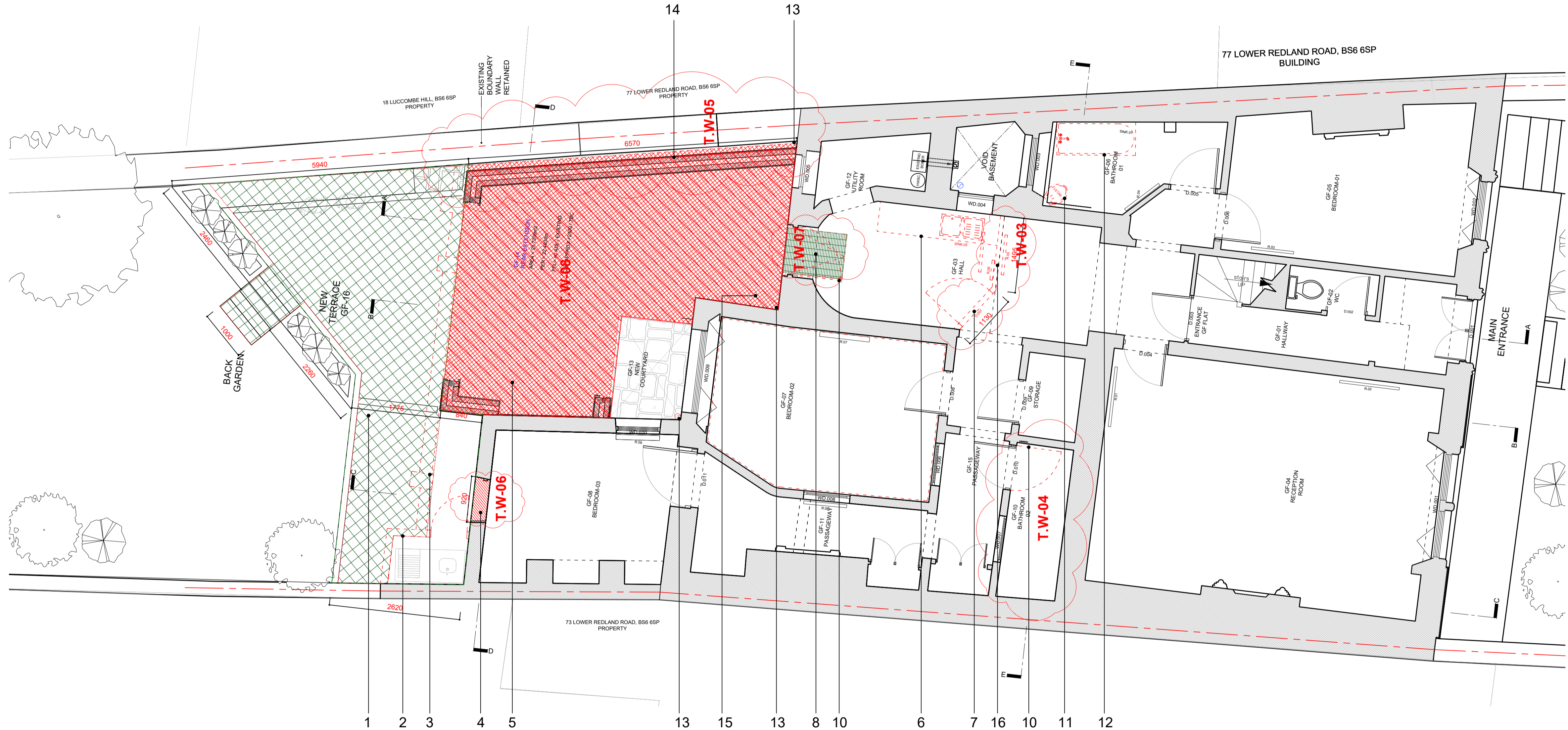
01-PROPOSED DEMOLITION GROUND FLOOR PLAN SCALE 1:50
