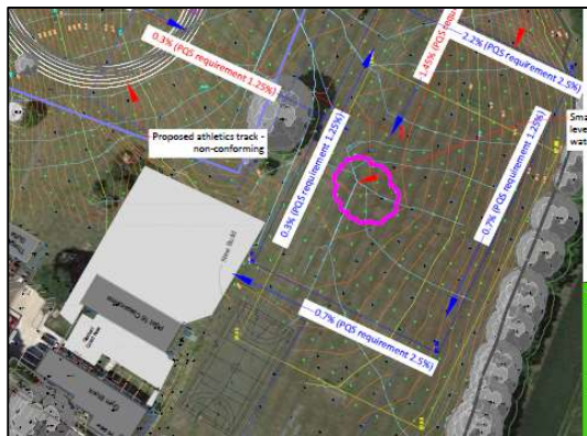
Figure 1 – area of localised undulation
