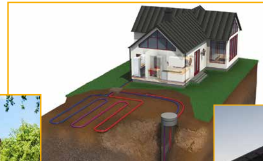
Ground Source Heat Pump (GSHP)
