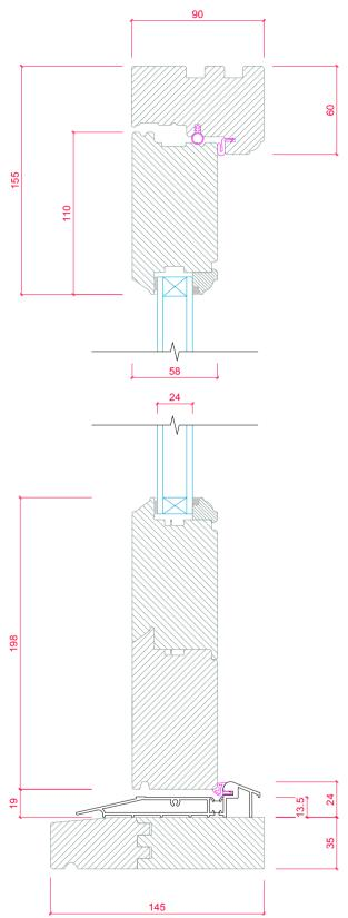
Optimal Door - Open Out Feature Mould: Ovolo Vertical Section Standard Threshold with 145mm x 35mm Projecting Cill
