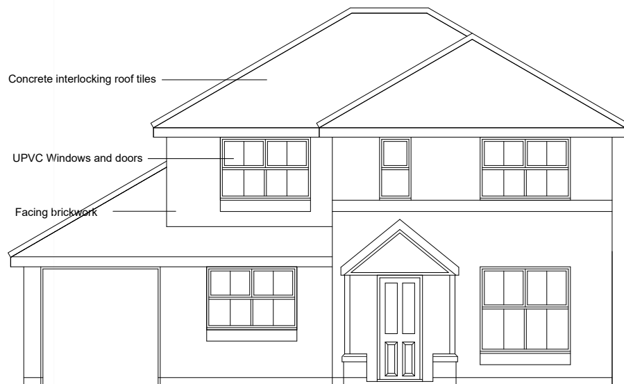
EXISTING FRONT ELEVATION
