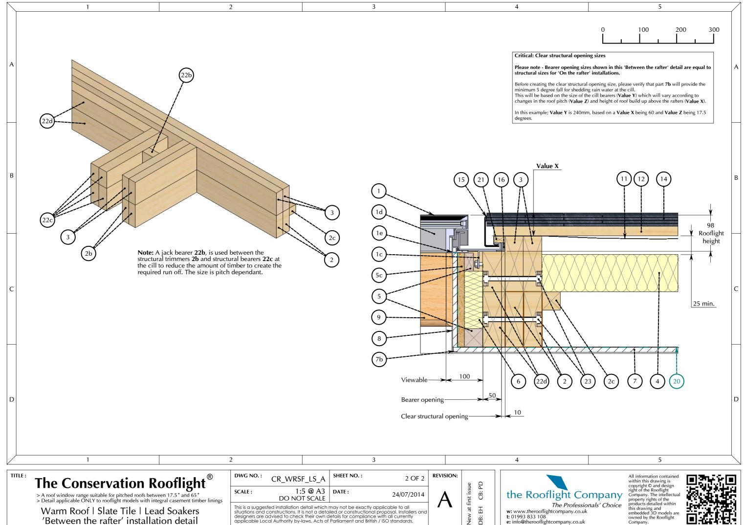
Warm Roof | Slate Tile | Lead Soakers 'Between the rafter' installation detail
