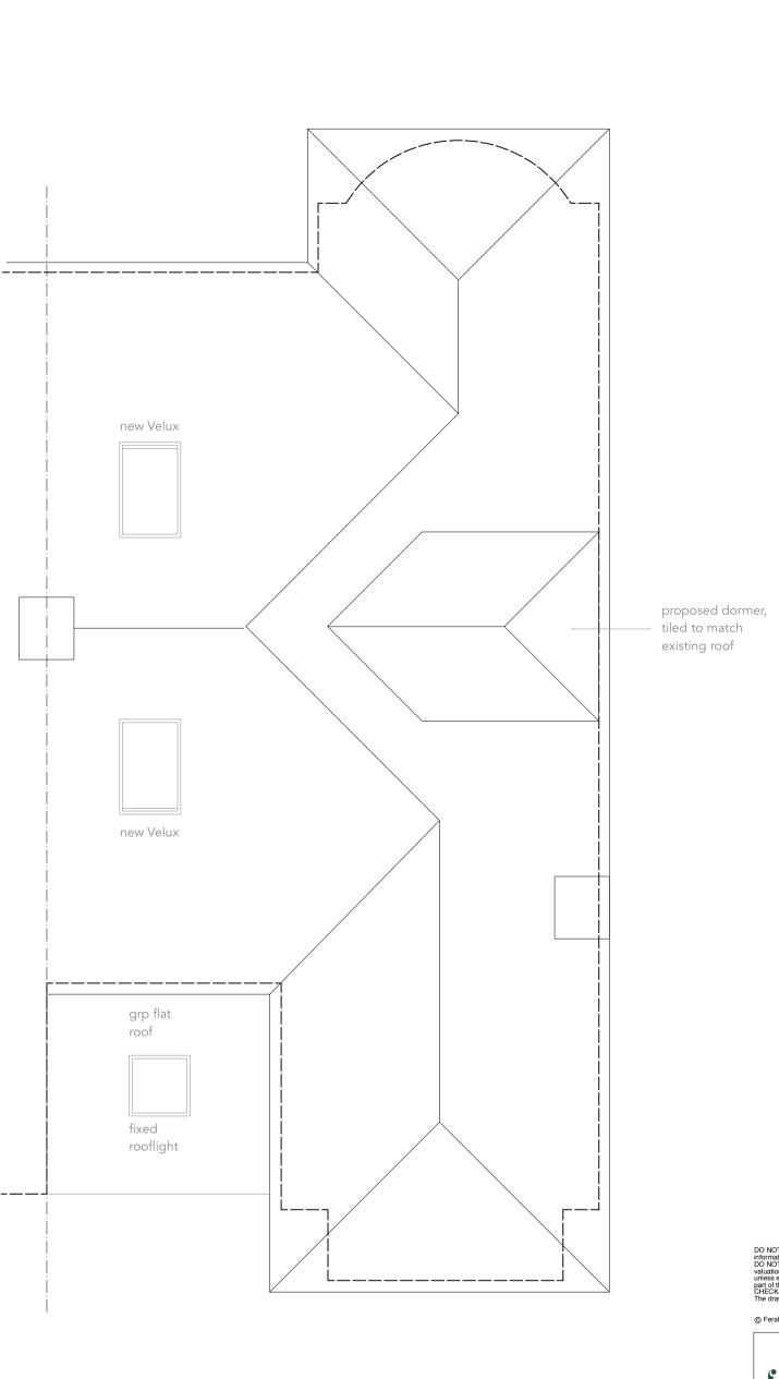
ROOF PLAN PROPOSED DO NOT scale from this drawing. DO NOT use any information without checking on site.
