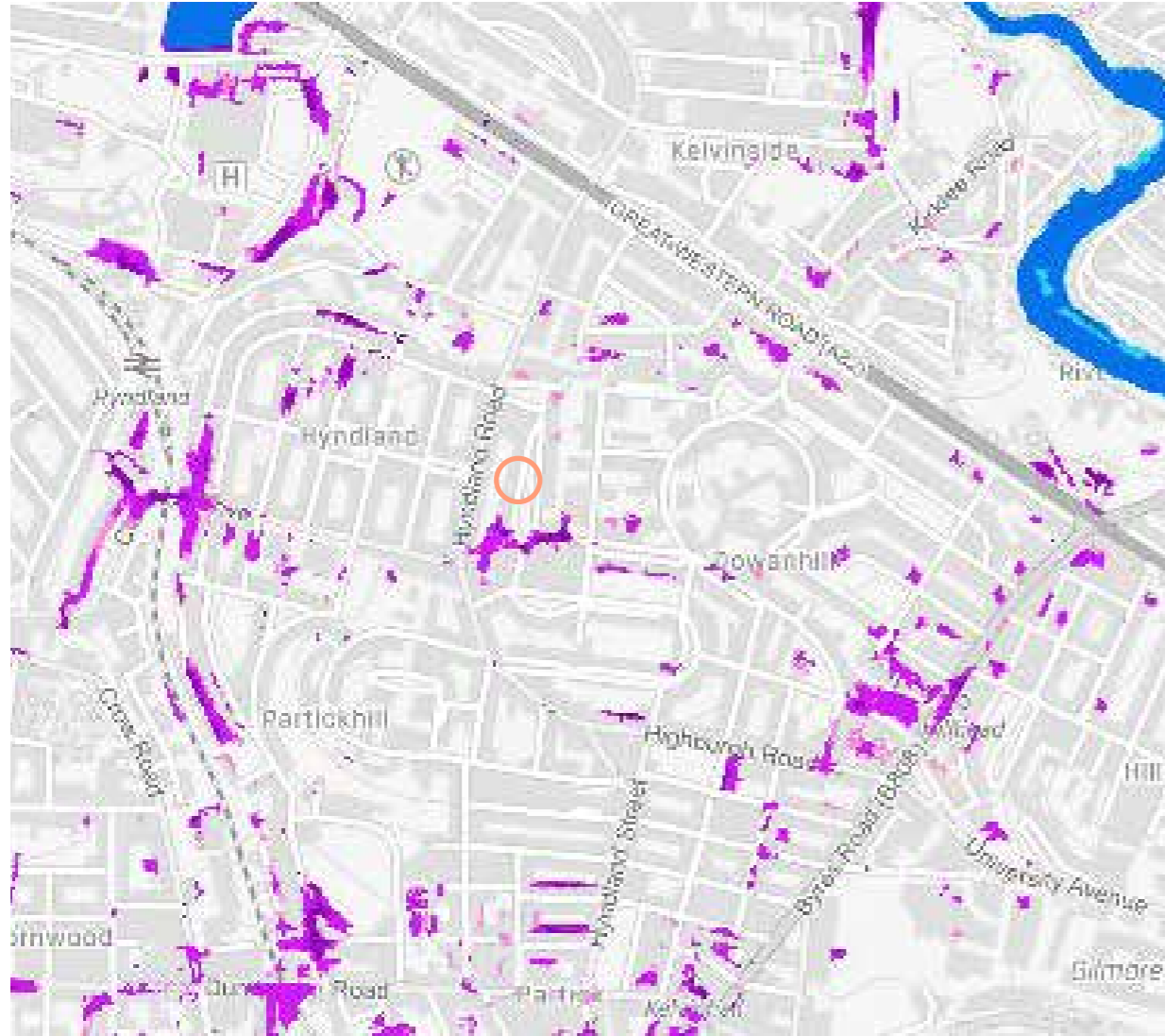
^ SEPA Floor Risk Map: site is largely unaffected with surrounding areas having some exposure to low rising surface water
