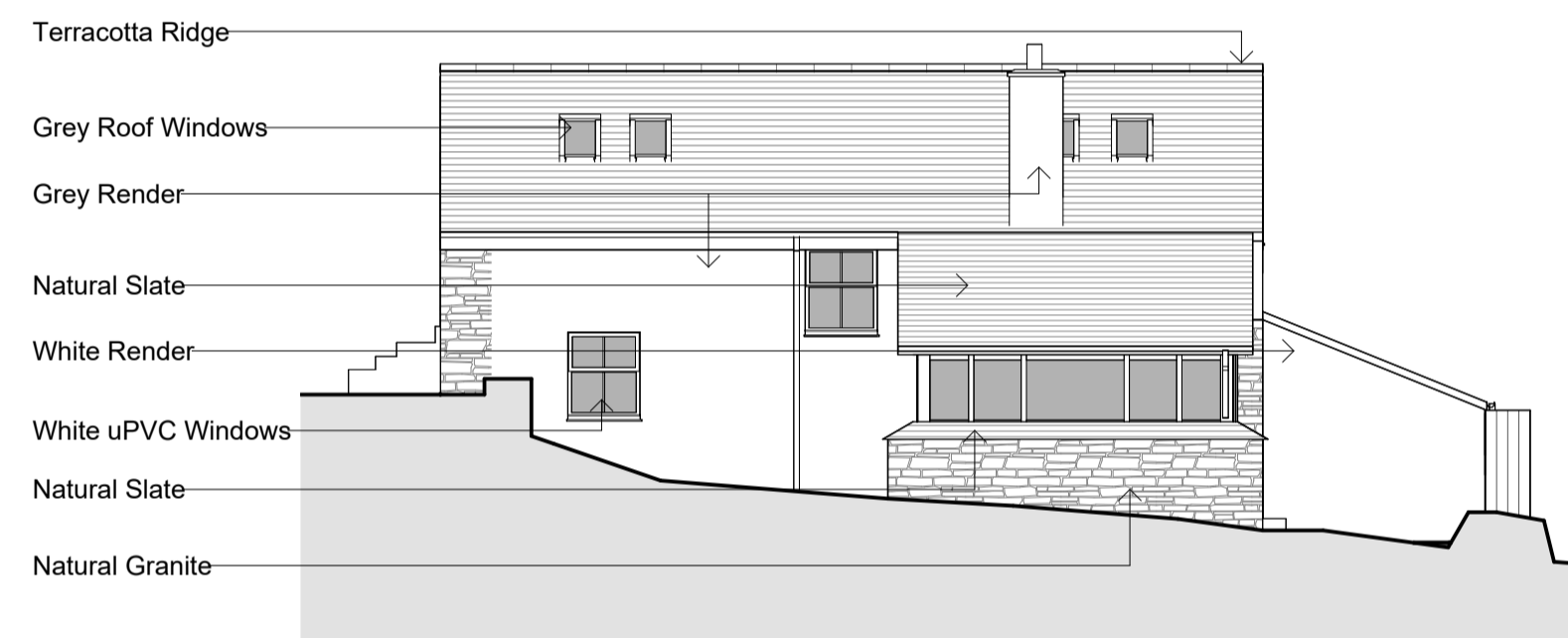
3 Elevation 3 - North East Elevation 1 : 100
