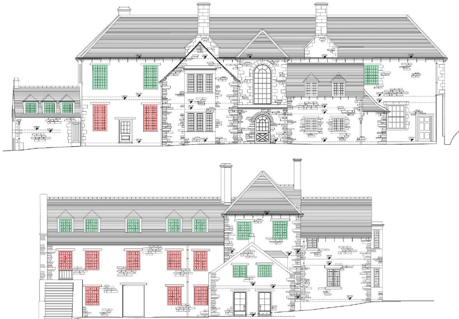
Figure 7 North (top) & east fronts (showing recently consented extension): historic casements; modern replica casements.
