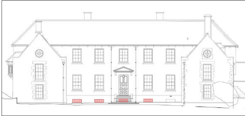
Figure 16 South front; basement windows (one behind entrance steps).
