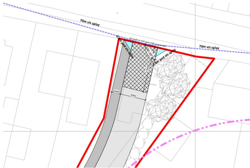
Figure 4 – Extract from Proposed Site Access Plan
