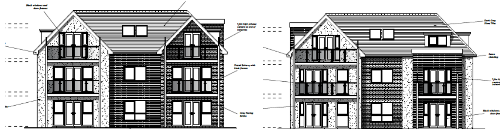
Proposed flatted blocks' front elevations
