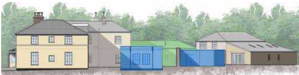
Figure 36 – Existing East Elevation – Proposed Demolitions
