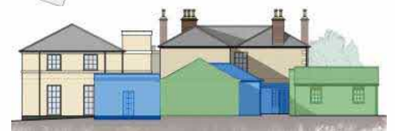
Figure 38 – Existing North Elevation – Proposed Demolitions
