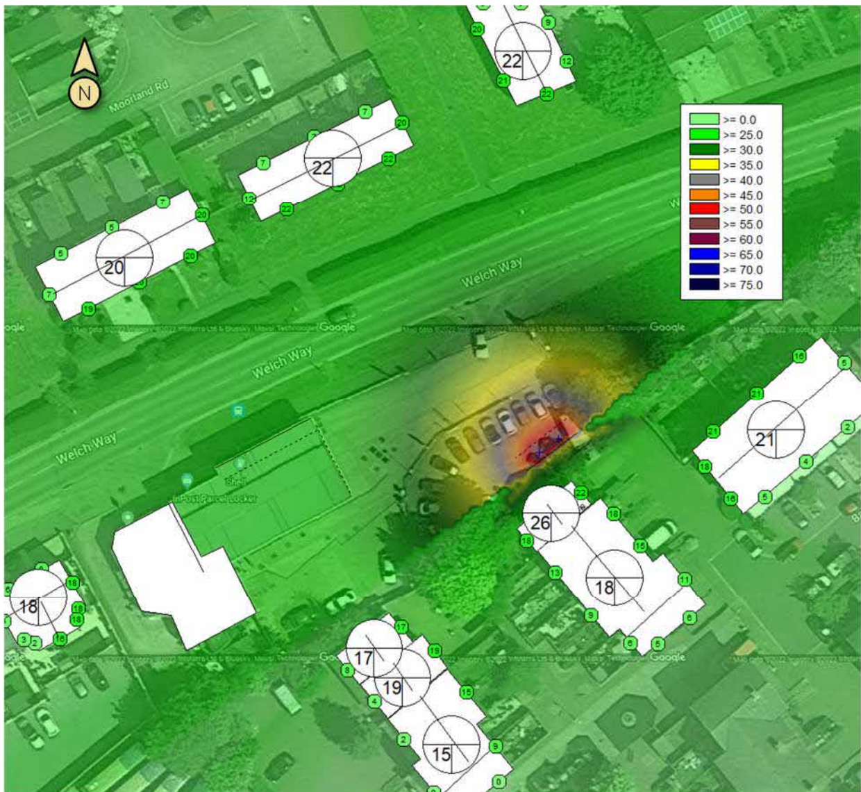
Figure 3: Worst case specific noise levels for all charging stations operating at any time
