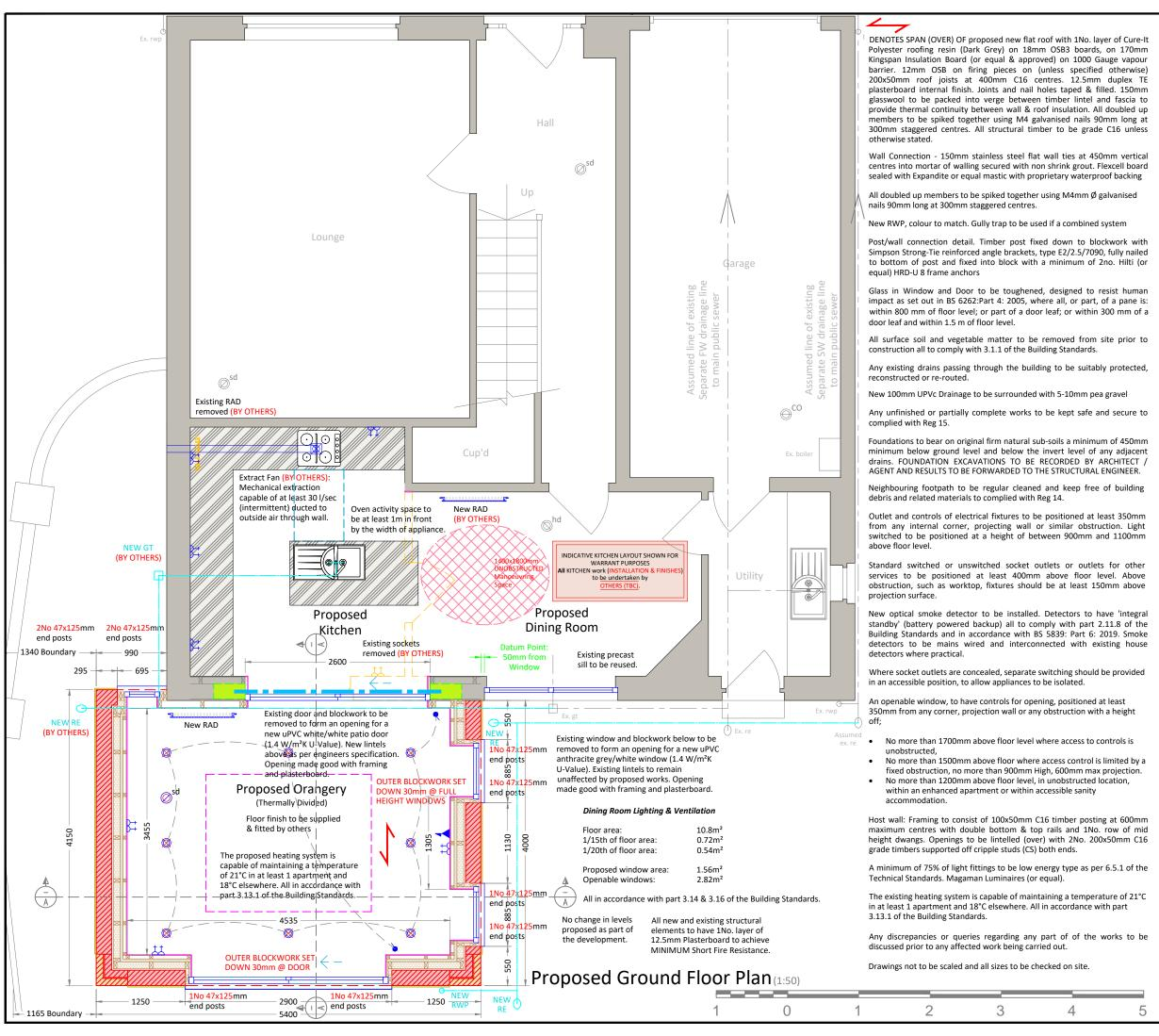
Final position of rad's to be agreed on site by customer. All new pipework insulated with foam pipe lagging to BS5422:2009. Rad fitted with thermostatic valve
