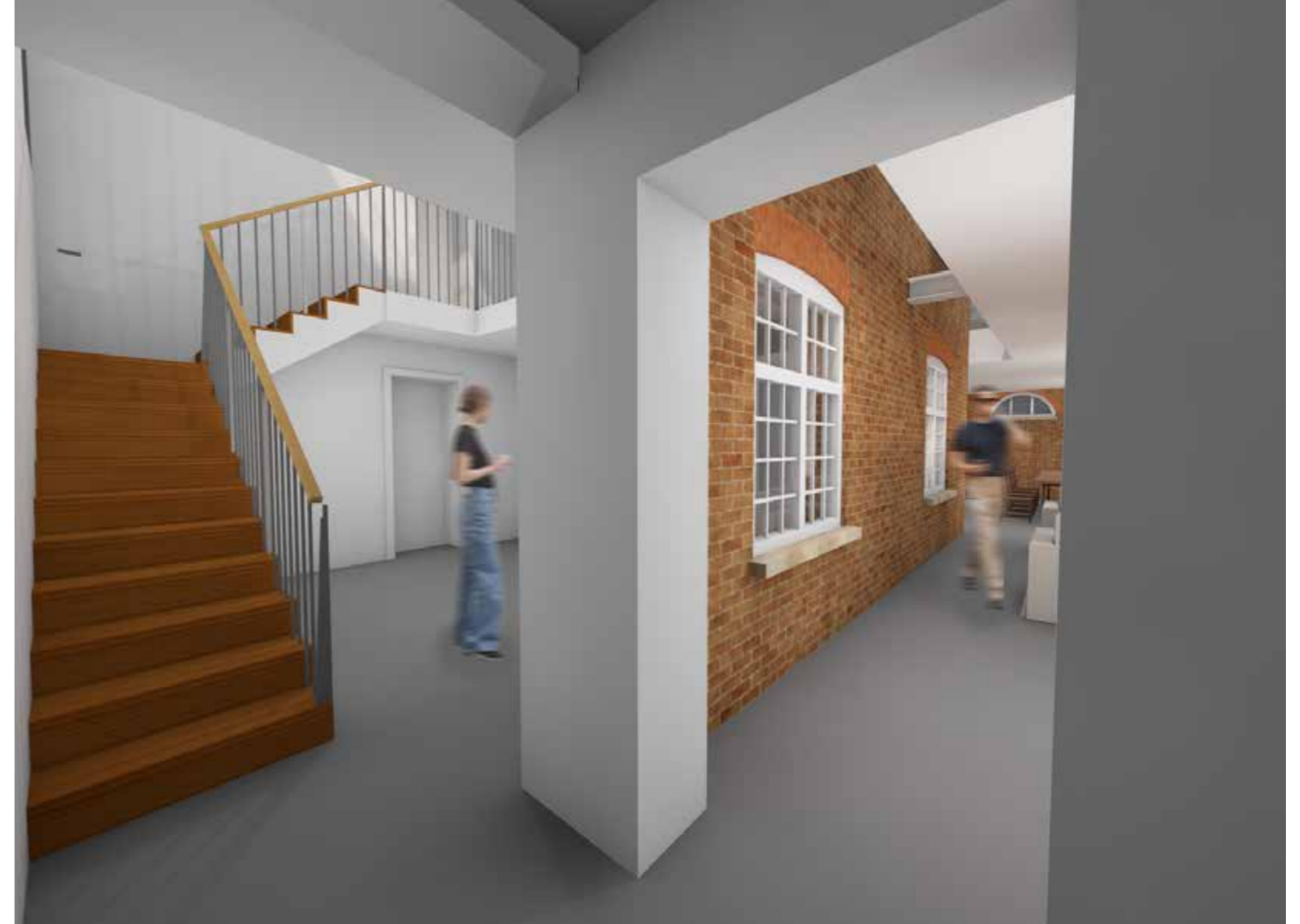
Sketch view from entrance lobby looking north-west. Existing windows and Flemish brickwork will be retained in situ to preserve character of the listed asset.
