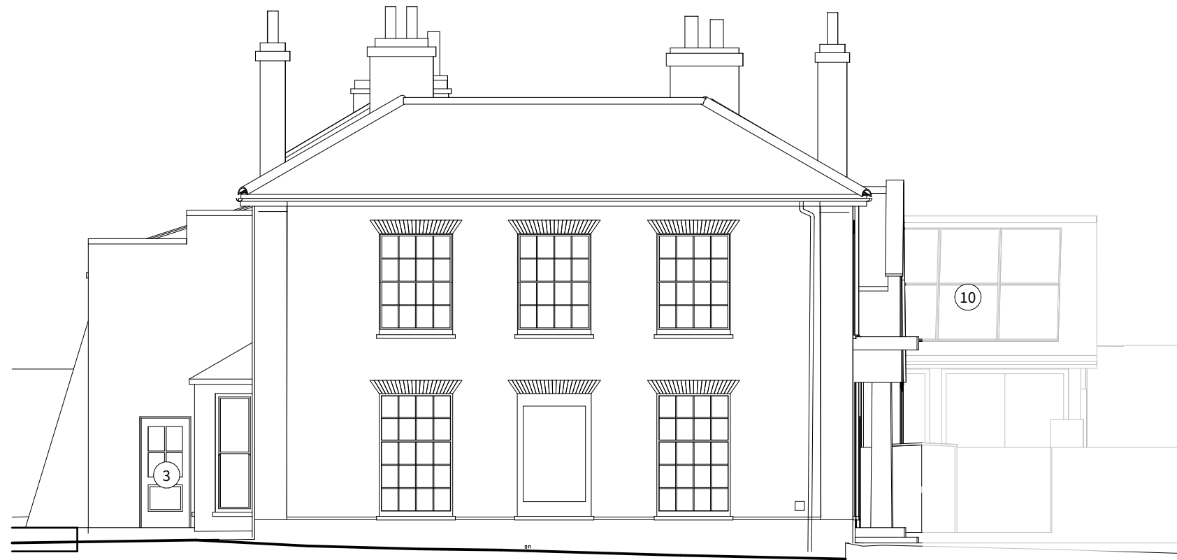
← Existing house and service wing; internal alterations and thermal upgrade works Existing stable block behind; internal alterations and thermal upgrade works → South Elevation (S1)
