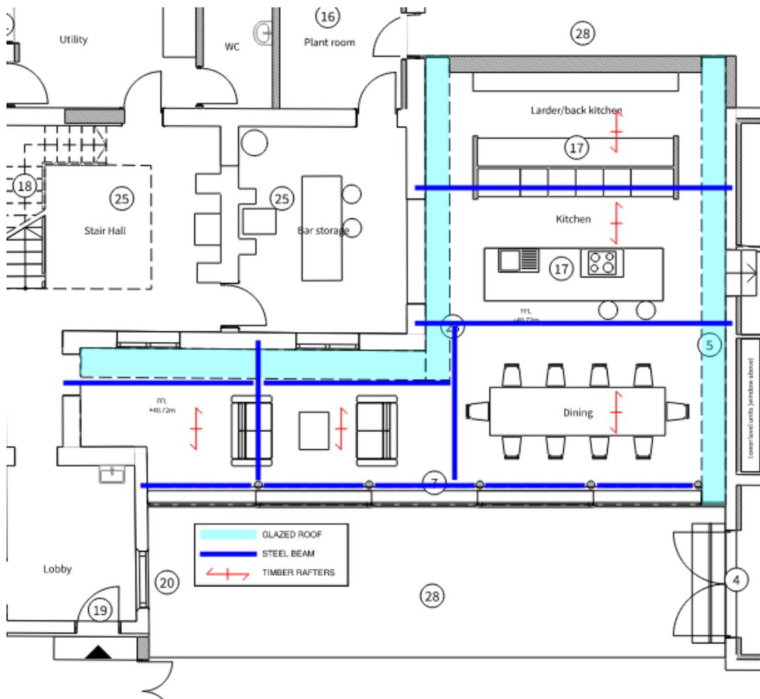
Figure 4 - Link roof structure
