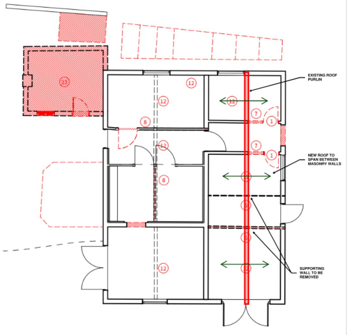
Figure 5 - Proposed stable block lean-to roof structure
