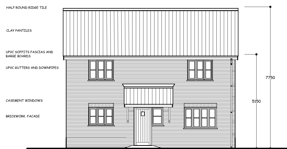
WEST FRONT ELEVATION - 1/100 scale PLOT no 5
