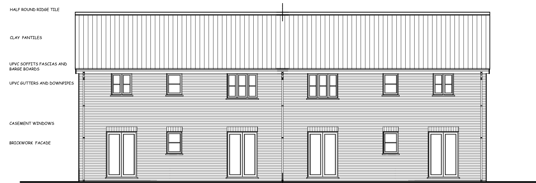
SOUTH REAR ELEVATION - 1/100 scale PLOT no 7 PLOT no 6
