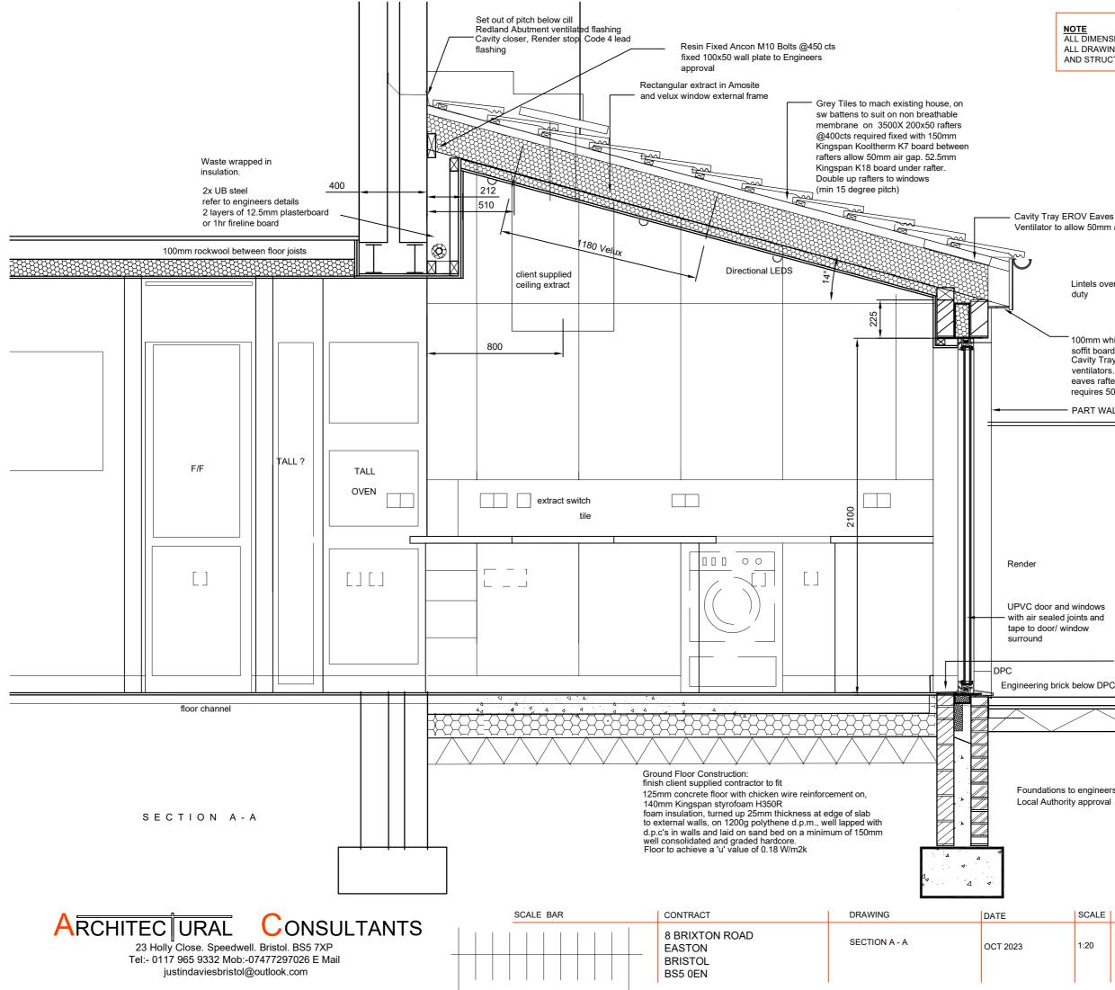
Cavity Tray EROV Eaves Roll out Ventilator to allow 50mm air flow.
