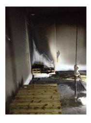
During test with some spread to covering of target crib
