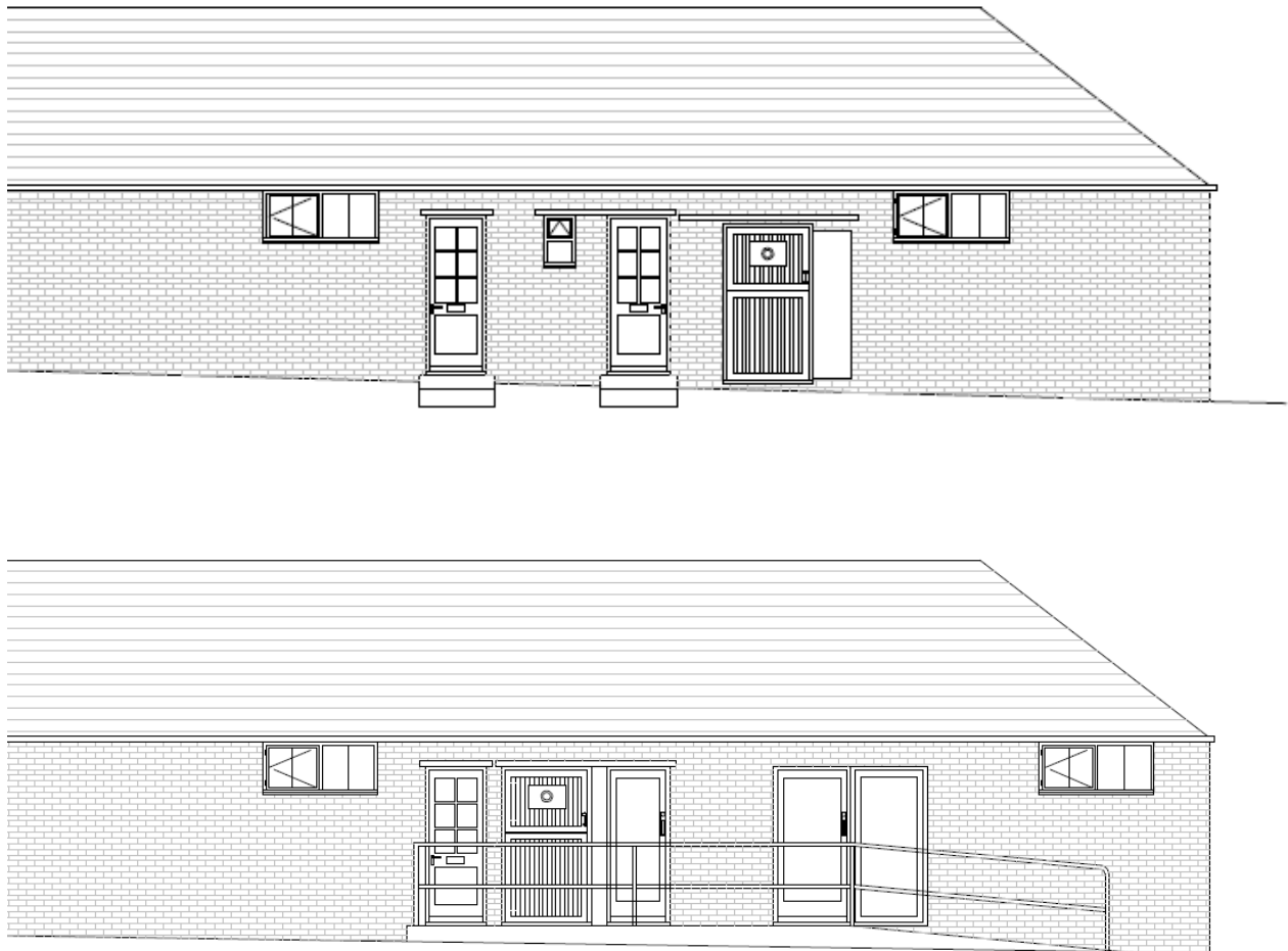
Figure 9: Existing (top) and proposed (bottom) eastern elevation
