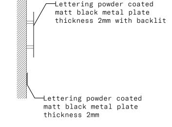
"WORK IN PROGRESS" lettering Each letter is 5 cm high Each letter is flat black metal plate thickness 2mm fixed to the building facade
