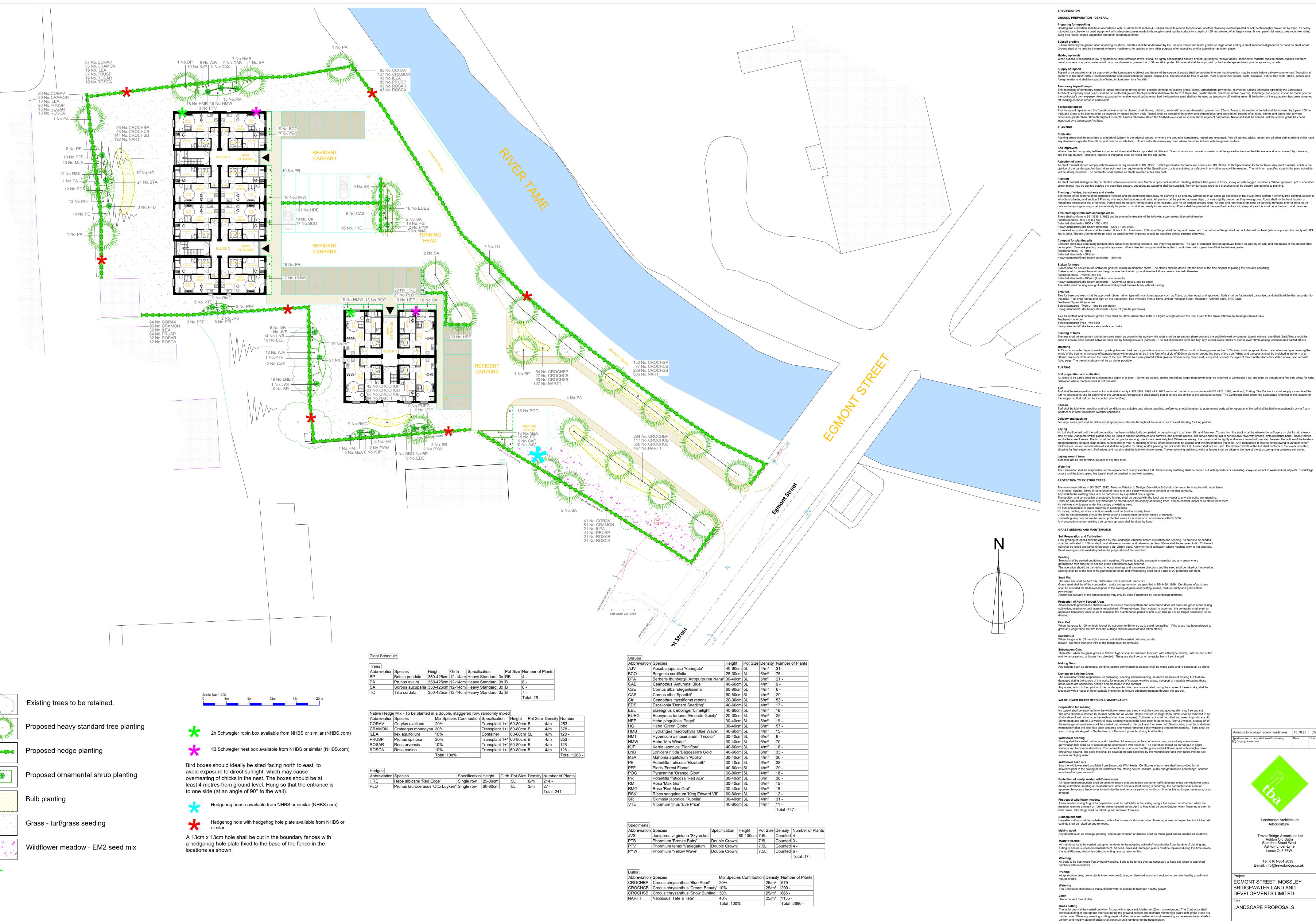
Grading and cultivation shall be in accordance with BS 4428:1989 section 4. Subsoil that is to receive topsoil shall, whether obviously overcompacted or not, be thoroughly broken up by hand, by heavy rotovator, by subsoiler or tined equipment with adequate passes made to thoroughly break up the surface to a depth of 150mm, cleared of all large stones, bricks, perennial weeds, tree roots (excluding
