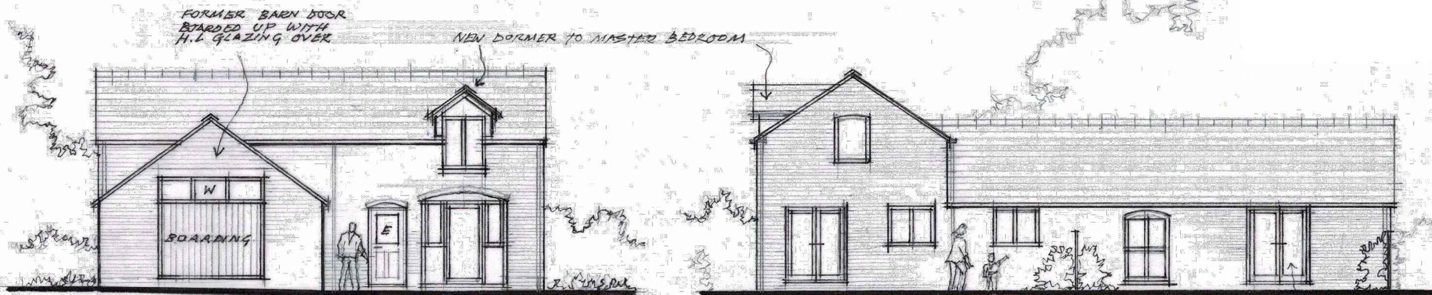
SOUTH ELEVATION AS PROPOSED. (EXISTING OPENINGS RE-USED)
