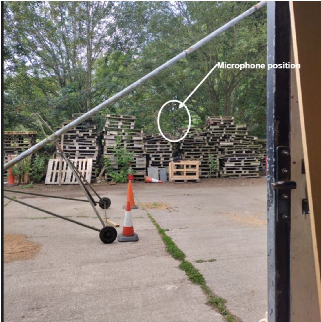
Figure 26 -- Specific sound level unattended measurement position
