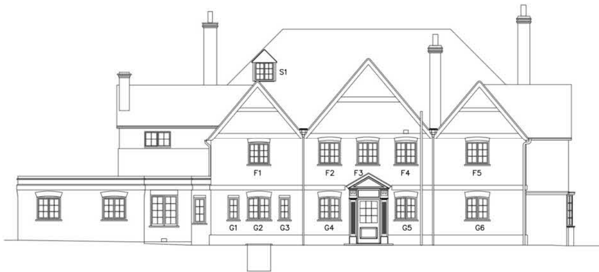
Figure 42: NW elevation window locations
