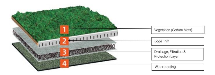
The BauderGREEN XF 301 sedum system has been designed to be a lightweight, single layer, green roof product. It enables green roofs to be installed on structures with very low weight loadings. Typically, the product is installed with BauderGREEN SDF mat to give adequate drainage.
