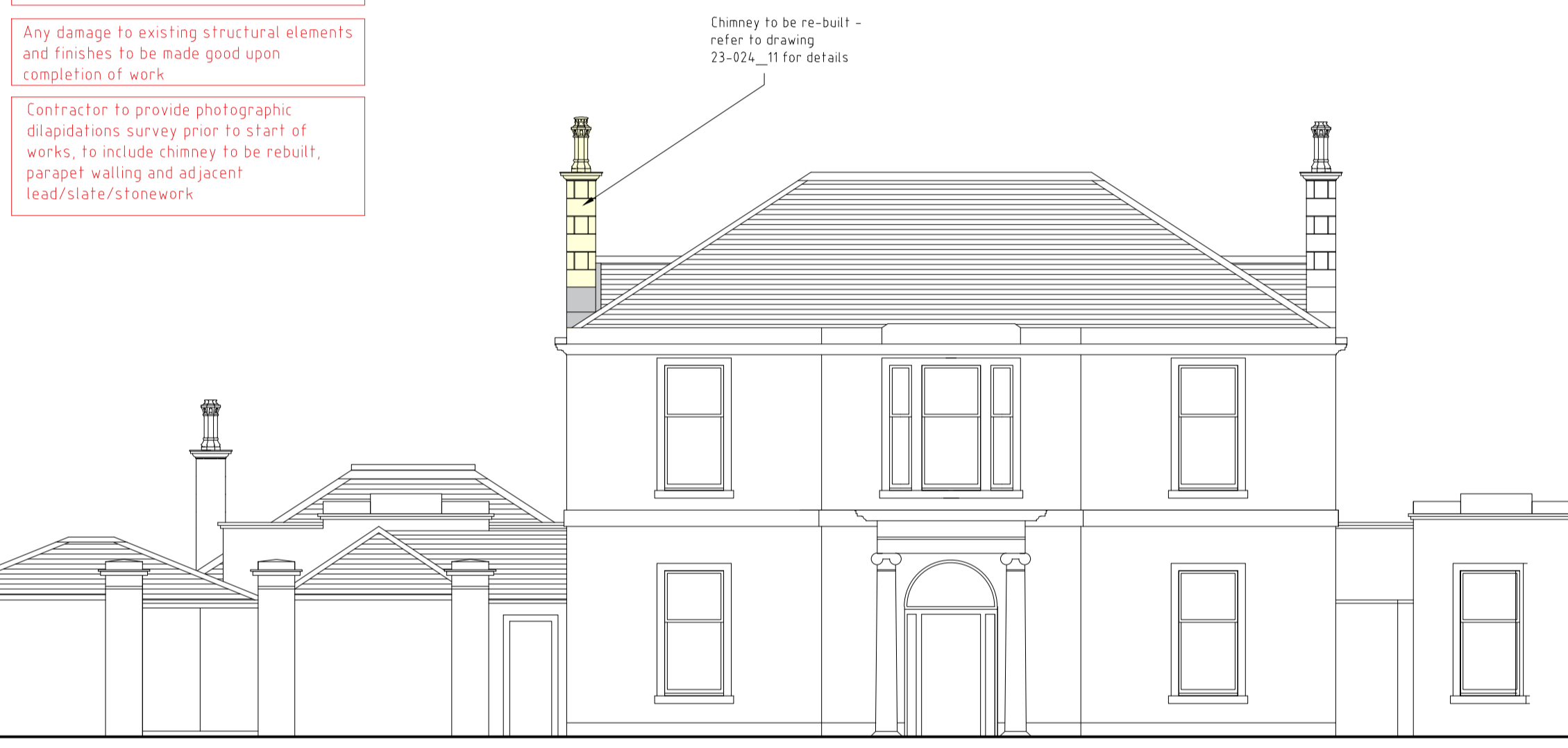
03 Front (North) Elevation - General Arrangement 1:100 @ A1
